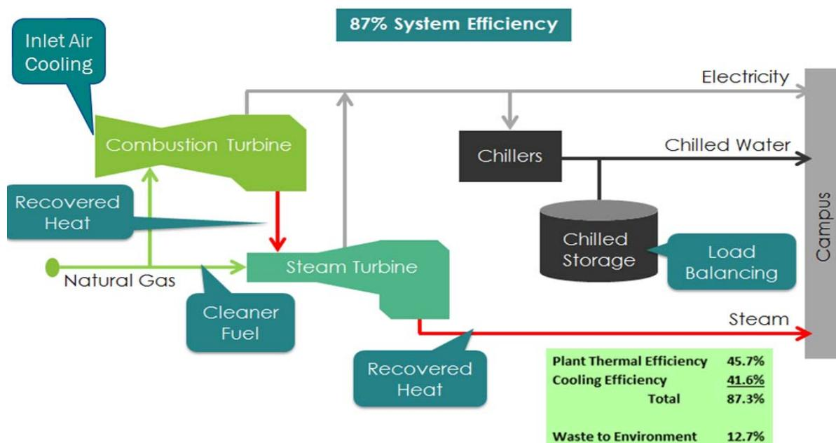
Waste heat from the combustion turbine is recovered to the steam turbine. The recovered heat is then extracted as steam for heating and hot water generation in campus buildings.
