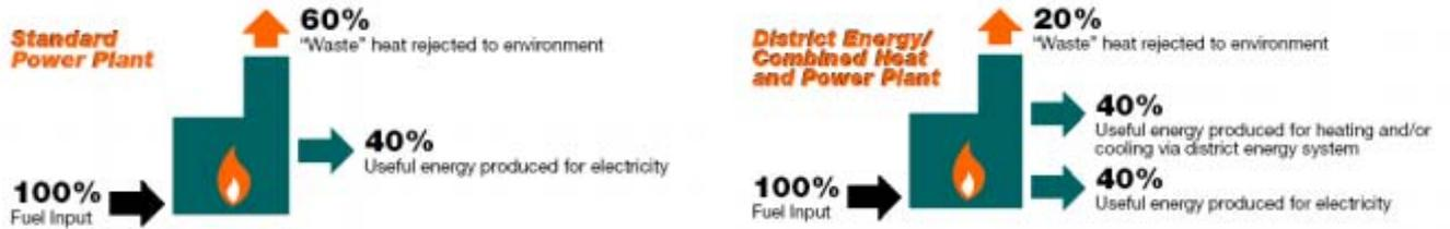
Energy efficiency comparison of a standard power plant versus a combine heat and power plant.
