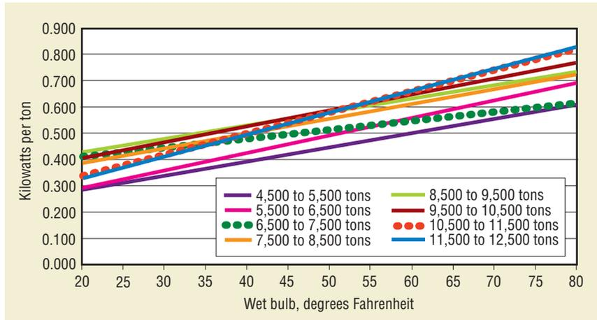
**FIGURE 4. The University of Texas at Austin Station 6 total plant performance (includes chillers, chilled-water and condenser-water pumps, and cooling-tower-fan energy).**
